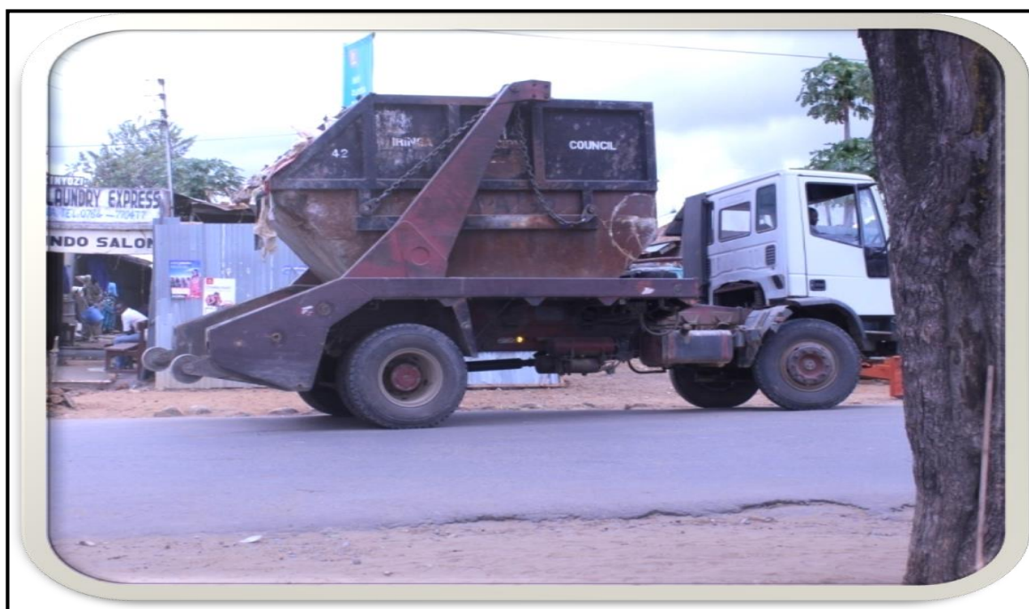
Plate 7.3: Vehicle used to carry skip basket
